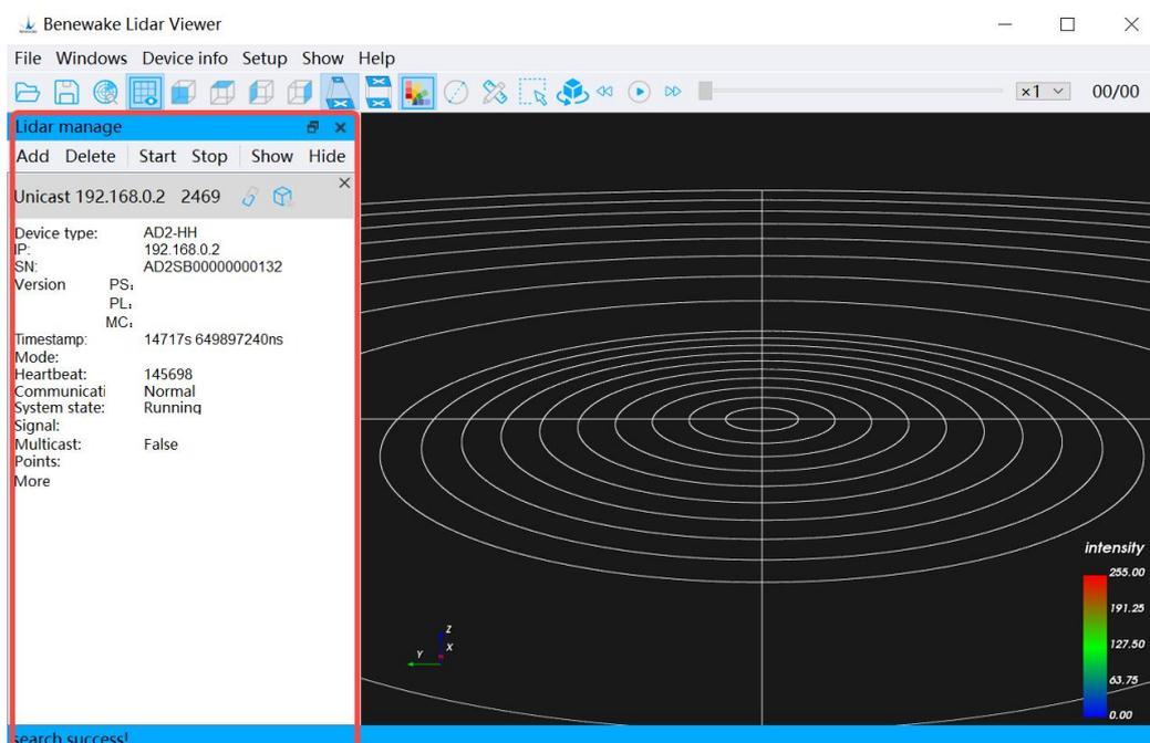
Figure. 7: Adding the device
