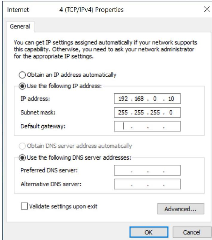
Figure. 1: Configuring IP address
