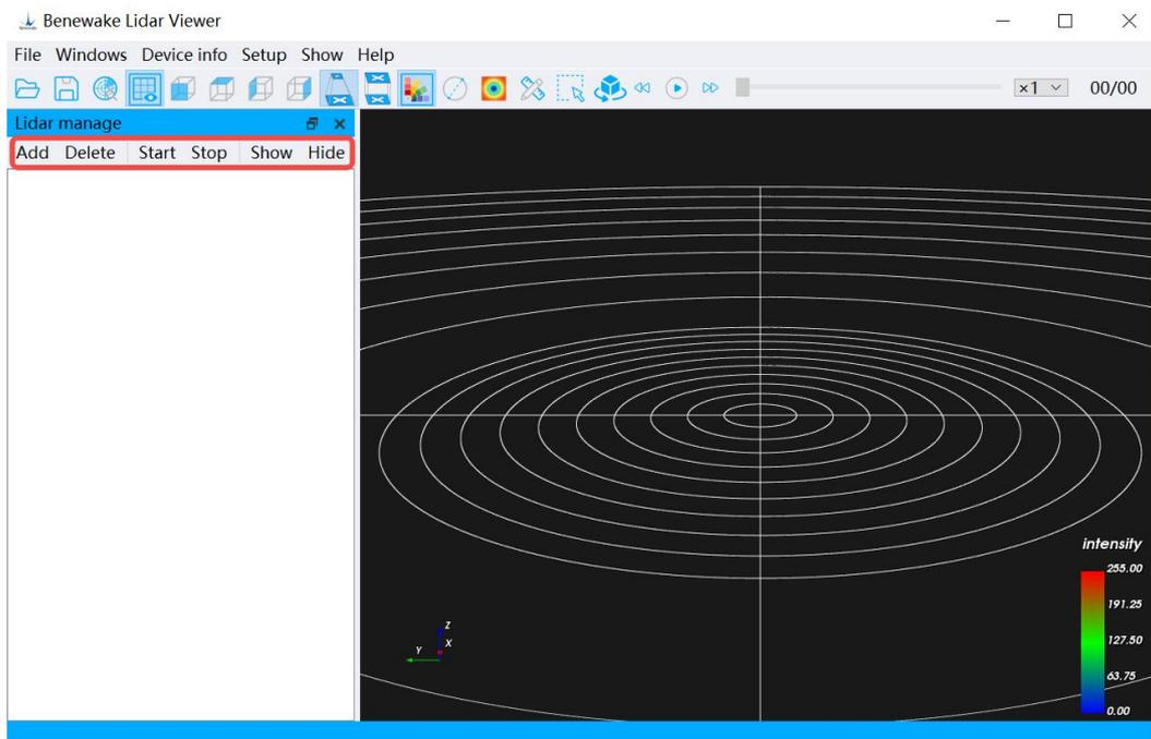
Figure. 21: Optional functions in device management bar
