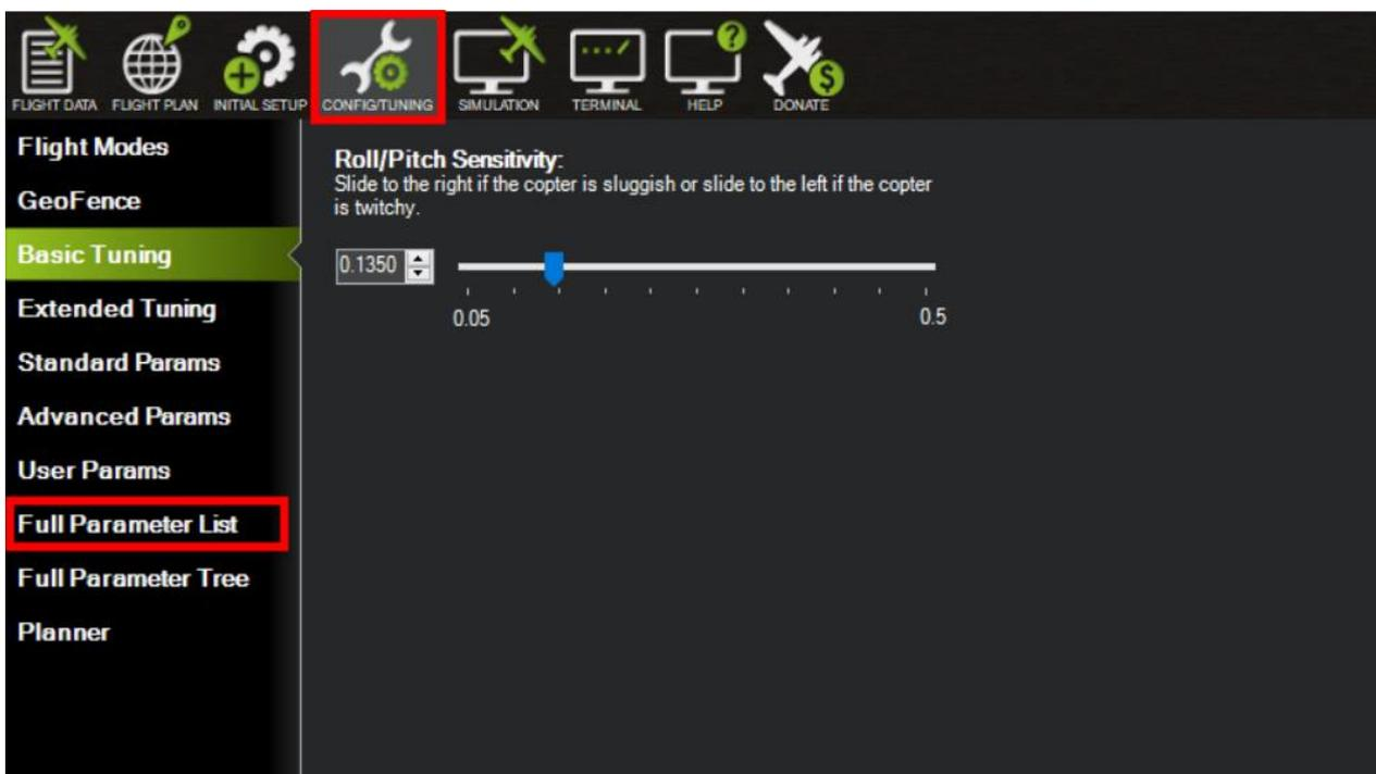
Upon setting of these parameters, click [Write Params] on the right of mission planner to finish. After writing the parameters, you need to power off the controller and then turn it on to apply the setting changes.
