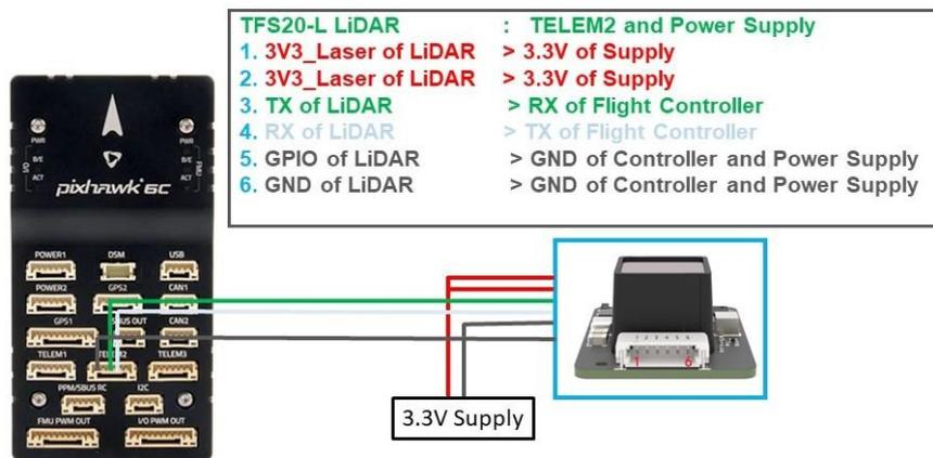
**Figure 3:** Schematic Diagram of Connecting TFS20-L with TELEM 2 Interface (Serial Port 2) of PixHawk 6C
